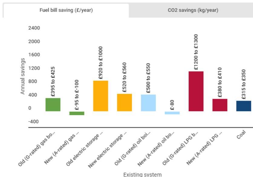
Figure 4: Potential annual savings of using an ASHP (EST)
